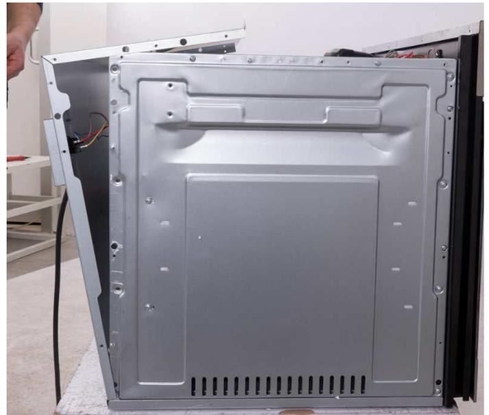
Remove the screws on the rear guard of the oven with a screwdriver. Release and take the rear guard off its tabs.
