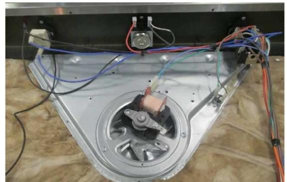
Remove the cables connected to the safety thermostat with a socket by holding on the terminals.
