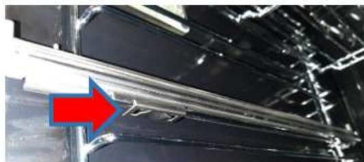
Telescopic rails are fixed by two clips at bottom side of part. You should open these clips locked by using a tool like screwdriver
