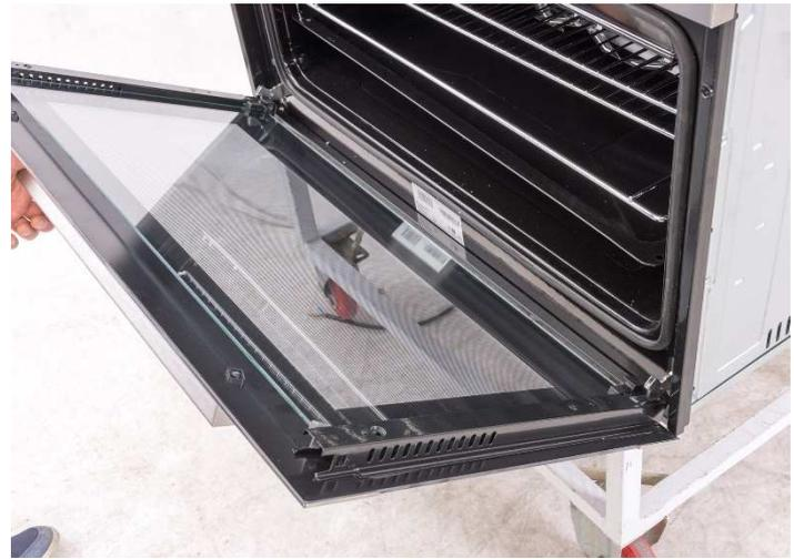
Open the front door. After opening the front door, open the clips locating on the front door hinge slot on the right and left sides by pulling them upwards.
