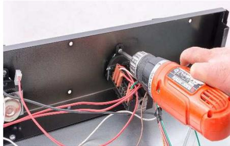
Remove the screw that connects the circuit breaker shell to the panel with a screwdriver.
