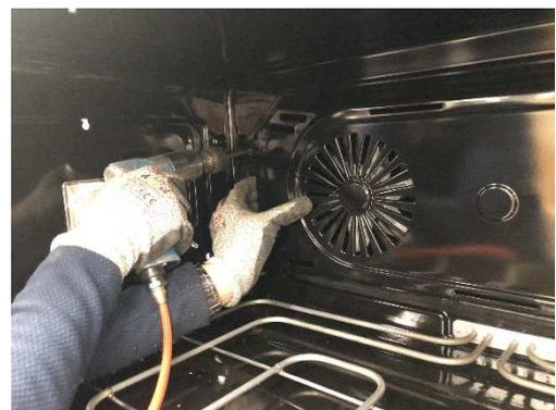
Remove the fan protection sheet by removing the screws with the help of a screwdriver.
