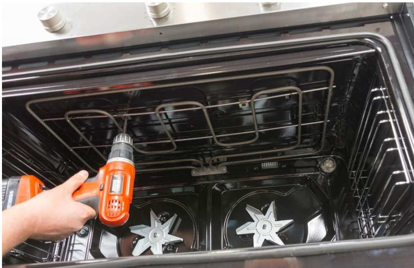
The heating element located on the upper side in the oven is attached to the chassis with two screws. Remove the screws with the help of a screwdriver. Then, the screw that secures the heating element to the chassis from inside must also be removed.
