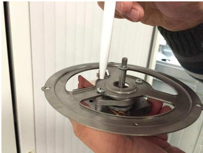
Remove the propeller before removing the motor assembly.
