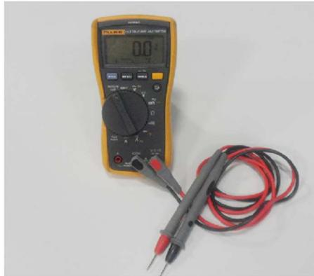
Multimeter set to heating element measuring position to measure the heating element value. If the heating element is OK, a heating element values appears on the multimeter.
