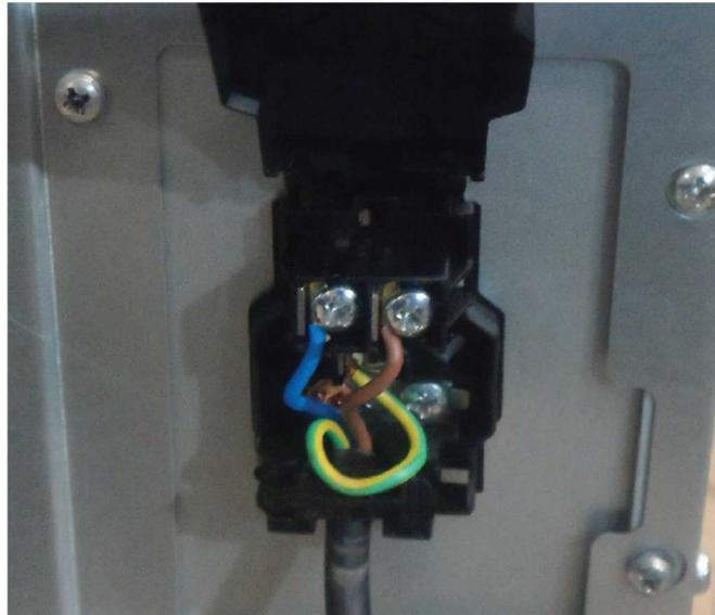
Grab and remove the oven inner power cables connected to the terminal from rear part by means of a nippers.
