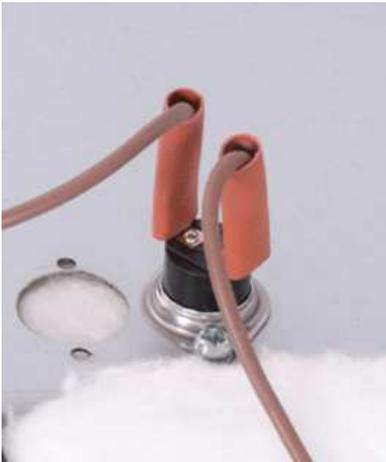
The purpose of the safety thermostat is cut off the phase or neutral before the oven temperature exceeds a certain value when the thermostat on the oven is short-circuited or due to continuous operation of any heater resulting from a short circuit. Since the point where the thermal cutter fitted on the oven is taken as the reference, the safety thermostat is expected to switch off only under abnormal conditions but not under normal conditions.
