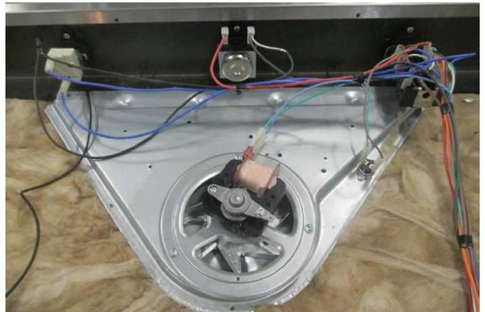
You can access circuit breaker, thermostat, mechanical/digital clock and cable connections after removing the service cover.
