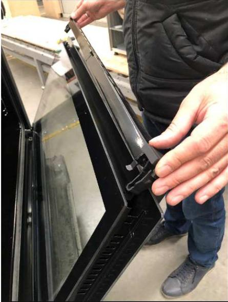
Remove the glass top profile by pressing right and left side after removing screws and plastic clips on side profiles.
