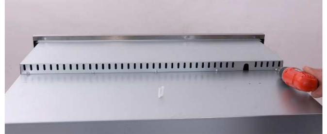
Remove the screws that connect the service cover of the product to the top cover.
