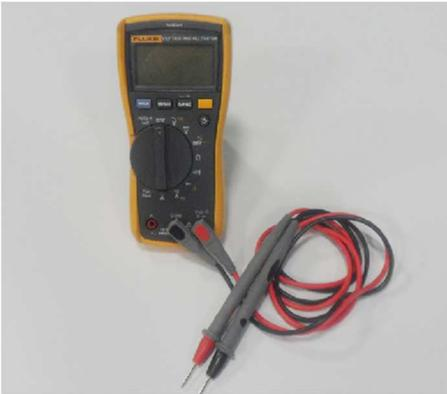
The current and power drawn by the components on the appliance is measured with a device called multimeter.
