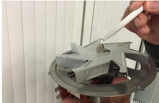
Remove the closed bolt to remove the propeller.
