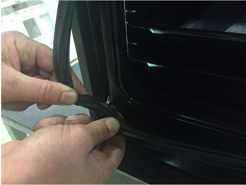
The tabs located on the sealing clamps on the chassis. You can replace the gasket by removing it from the tabs.
