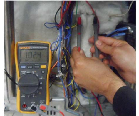
If any value appears on the multimeter screen, it means the heating element is in operating status.
