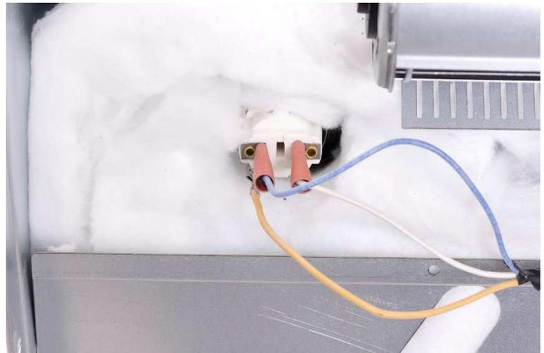
Pull and remove the cables attached to the lamp located behind the chassis from their terminals to replace the oven lamp. You can remove the lamp cleared off the cable connections by pressing the tabs.
