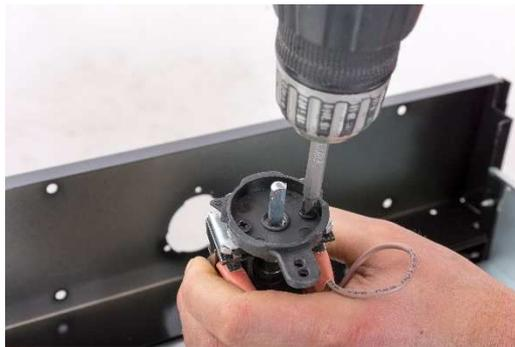
Remove two screws that secure the circuit breaker to the circuit breaker shell with a screwdriver.
