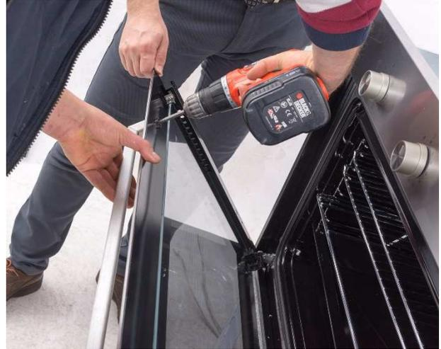
Remove the screws on front glass.
