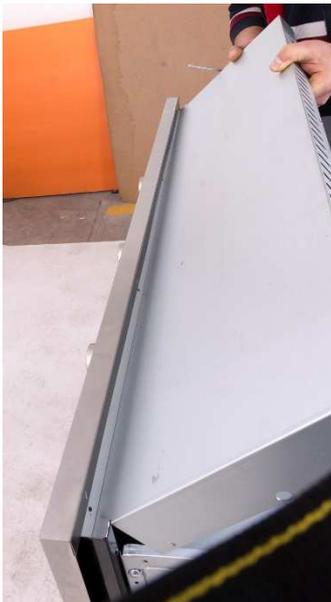
Lift the rear side of the service cover up with an angle of 30° and push it to the rear side of the oven to remove it
