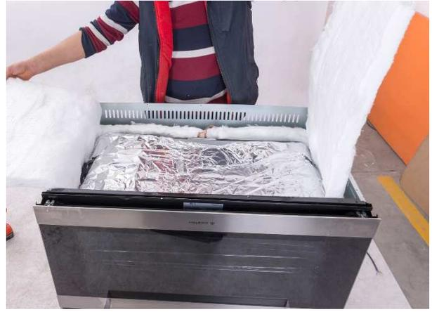
Remove the wire of the insulation coiled around the chassis with wire.
