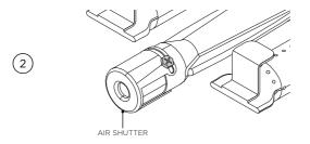
With a screw driver, loosen the lock screw on the face of the air shutter so it can be adjusted. If the flame is yellow turn the air shutter counter-clockwise, if the flame is noisy and tends to lift turn the air shutter clockwise.
