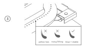
Reinstall the U-burner and light to check. If the flame is blue and stable, remove the burner, tighten the air shutter screw and replace all parts. If flame is still unstable, repeat the above steps.
