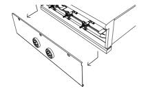
Pull the valve panel down then outward and unplug any wires.
