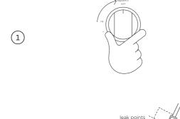
Prepare soap solution by combining one part liquid detergent and one part water. Pour into a spray bottle. Ensure all control valves are in the **OFF** position before turning the gas supply **ON**.
