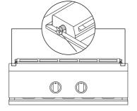
Using a match extension rod, carefully light a match and hold up against the base of the flash tube as shown.
