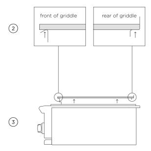
Grip the griddle plate from under the brackets at the front and rear of the product as shown.
