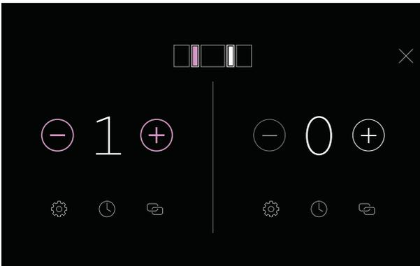
2. Press  $\ominus$  or  $\oplus$  to adjust the fan speed. There are 5 speeds plus **BOOST**. Press and hold  $\ominus$  or  $\oplus$  to jump to 0 or **BOOST**, respectively.
