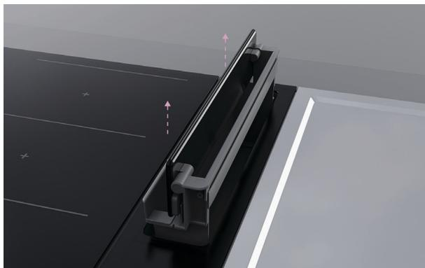
1. Open downdraft cover. Lift filter box by the cover to access the filter and downdraft cavity. Clean the cavity with a damp cloth and mild detergent.
