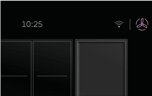
1. Push the downdraft cover lightly to open. Press
