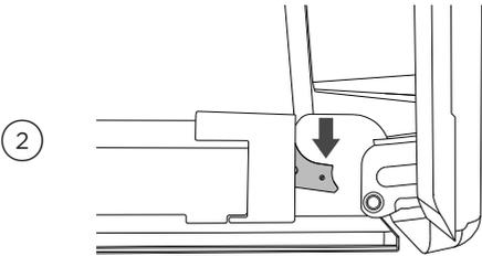
Ensure the door is firmly in place on the hinges. Open the door fully again and push each locking lever down to lock the door onto the hinge.
