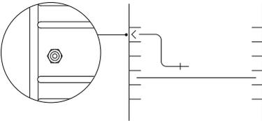
Place food in the oven and plug the probe into the socket inside the oven, on the left hand side.
