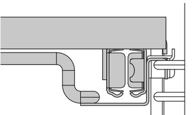
Ensure sliding shelves are positioned on top of the side rack wires instead of between them.
