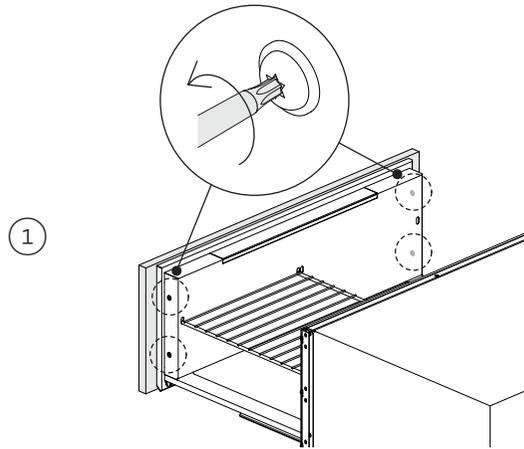
Open the drawer fully, and slightly loosen the T20 star head machine screws.
