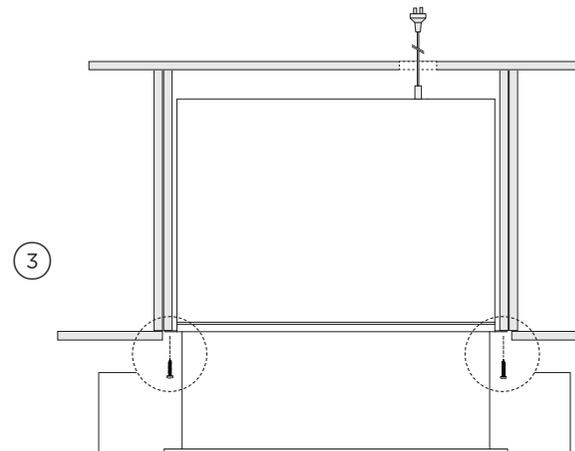
Open the drawer and secure the attachment flanges of the drawer to the side edges of cabinetry with T20 star head machine screws.
