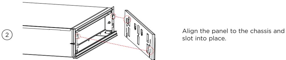
Align the panel to the chassis and slot into place.
