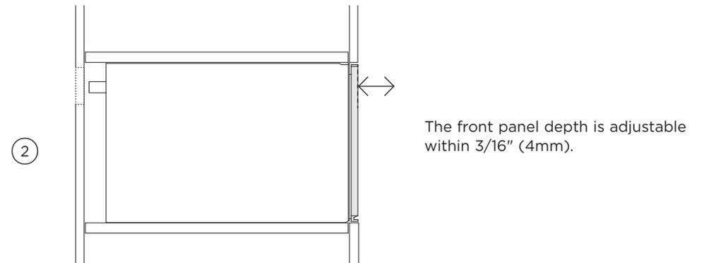
The front panel depth is adjustable within 3/16" (4mm).
