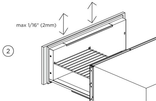
Adjust to the required height and then re-tighten the screws. The height is adjustable within 1/16" (2mm).
