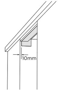
Align the supplied moisture protection tape to the cabinetry as illustrated
