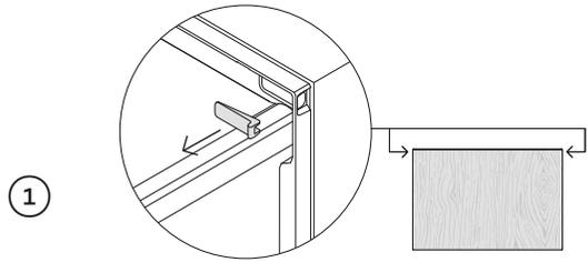
1 Partially open the drawer and remove the first screw cover from the trim moulding.
