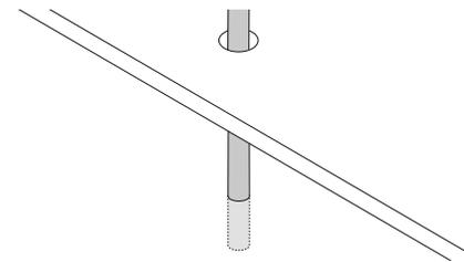
Route the venting hose through the floor. Ensure any excess hose is removed.
