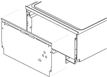
Carefully pull the bracket down and out from DishDrawer™ Dishwasher and unplug the Knock-to-Pause module and earth wire.
