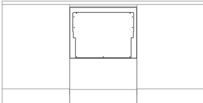
Push the product into the cavity, pulling the hoses through as you push to avoid crushing or twisting them.
