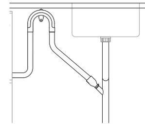
Pull the hose through the drain hose support before threading the wire clip on to the hose and fitting to the supplied hose joiner. Secure using the wire clips. Ensure hose is routed straight to the joiner, removing excess drain hose if necessary. Do not shorten the inlet hose. Unplug or drill out the waste tee before securing joiner to sink trap or waste tee.
