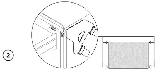
2 Secure to cabinetry via the brackets. Pre-drilling a pilot hole may be required depending on the cabinetry material.
