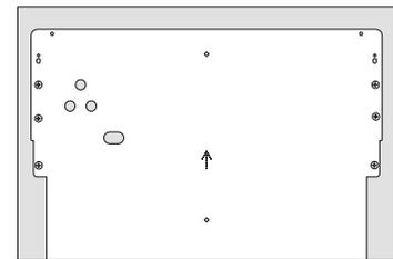
Secure the bracket to the panel using a minimum of 3 screws on either side.
