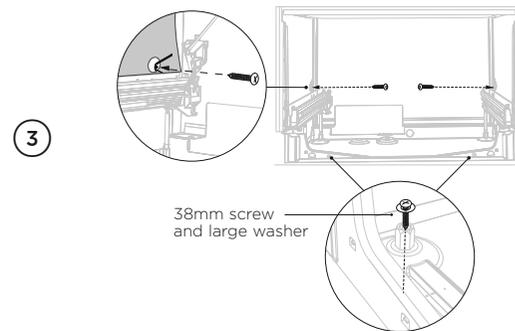
3 Secure to cabinetry via all three fixing locations in the chassis. **Ensure sound insulation is replaced correctly.**
