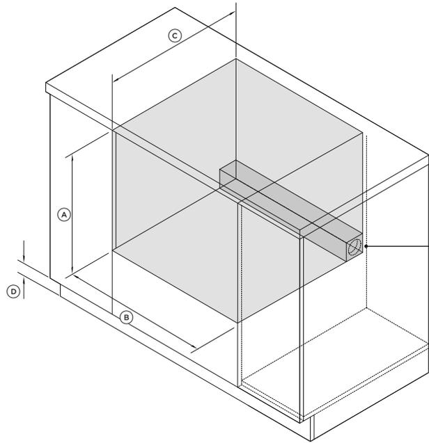
Connections can be located in an adjacent cabinet on either side of the DishDrawer™ Dishwasher\*\*\*
