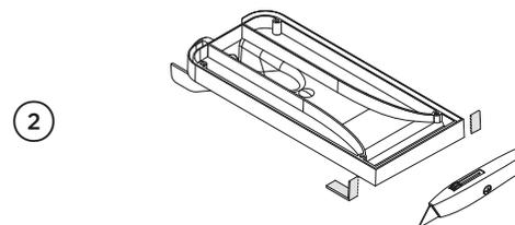
On a protected surface, carefully cut and remove the clips from the vent as shown. Refit the top cover.
