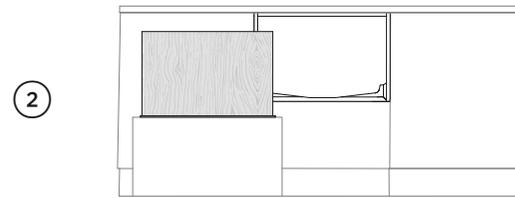
2 Lift the drawer off the runners and carefully set aside on a protected surface. Push runners back in. Take care not to pull drawer out too far to prevent any strain on the hoses. Where possible, protect the base of the tub to prevent damage.
