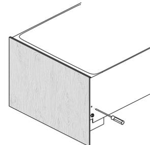
Insert a Phillips screwdriver into the hole above the side pin and rotate to adjust the panel alignment. There is a maximum travel distance of  $\pm 2\text{mm}$ . Repeat on the other side if required.
