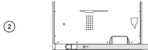
Push the vent hose onto the elbow firmly to secure.
