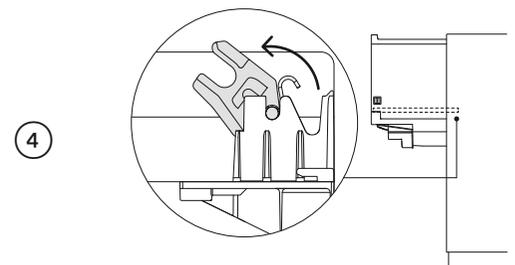
4 Before refitting the drawer, ensure the hoses are not twisted. Refit the drawer to the runners and clip into place via both locking tabs.
