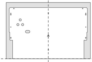
On the back of the panel, mark the centre and align the base of the bracket with the base of the panel.
