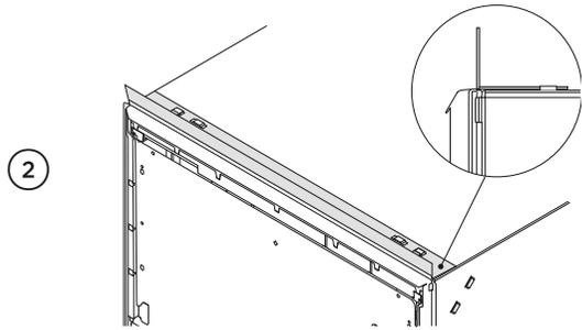
Check the trim seal is facing forward and sitting flat under the bracket.
