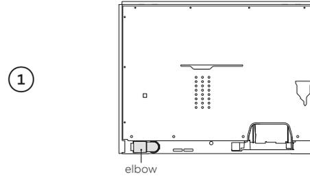
Rotate the elbow at the rear of the product to either the left or right depending on your venting location.
