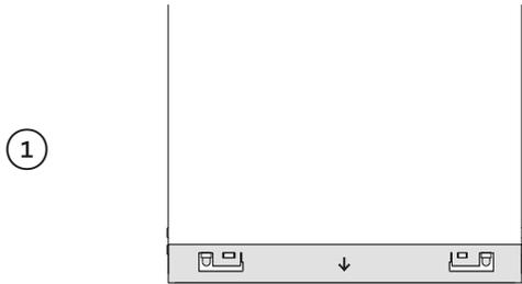
Align the bracket to the chassis ensuring the arrow is facing forward and firmly slot the tabs into place to secure.
