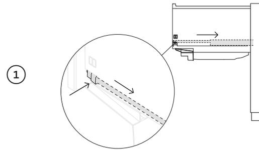
1 Open the drawer and press both locking tabs back to release.
