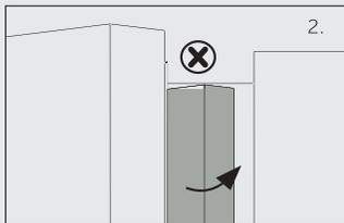
If you try to close the left door and the vertical door strip is unbent (2), you should bend it firstly, otherwise the door strip will hit the fixing shaft or right door. Thus a damage to the door slip or a leak will occur.
