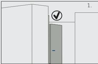
When you close the door, the vertical door strip on the left door should be bent inside (1).
