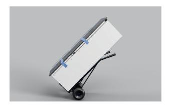
Keep the appliance at a 45° angle when shifting. Tilting more than 45° can damage the refrigeration system.
