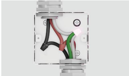
Connect the factory-taped green and white oven wires to the neutral (white) wire in the junction box.
