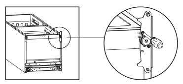
5. Adjusting the hinge core position of the lower hinge and upper hinge to opposite position
