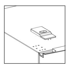
3. Take off the upper door, take out the screw from the middle hinge by cross screwdriver, then take off the lower door.
