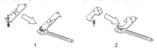
6. Install the lower hinge under to the refrigerator like below, screwing in the adjusting feet, make sure the position in horizon.
