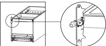
7. Install the lower door, adjust and fix the middle hinge onto the cabinet.
