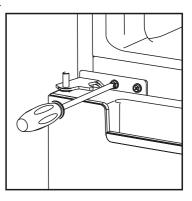
8. Place the upper door back on. Ensure the door is aligned horizontally and vertically so that the seal are closed on all sides before finally tightening the top hinge. Then inert the top hinge and screw it to the top of unit and then fix hinge cover (in accessary bag) by screw.
