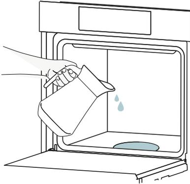
1. Remove all racks, trays and side racks from the oven, then pour 100 ml of water into the base of the oven.
