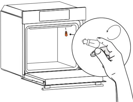
2. Unscrew the light bulb to remove it. Replace with a new bulb and refit the protective cover.
