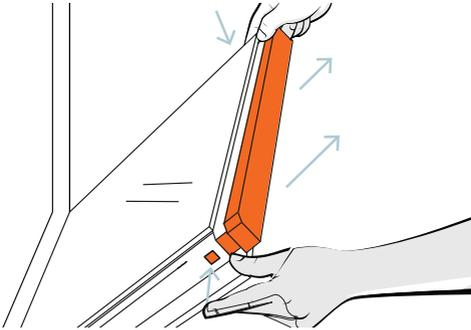
1. Shut the door halfway, then press the buttons on both sides of the door at the same time to release the cover on top of the door.
