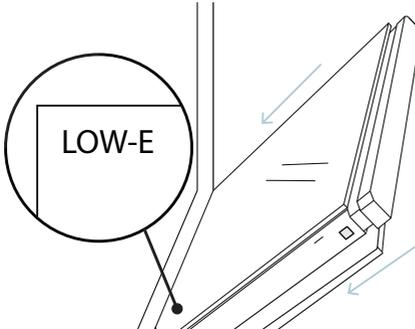
3. Once clean, carefully refit the panes and ensure the 'LOW-E' label of the middle pane, and the 'PYRO' label of the inner pane, are positioned correctly in the lower left-side corner of the door.
