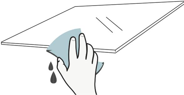
2. Carefully remove the inner and middle panes and wipe clean with a soft, damp cloth and mild detergent.
