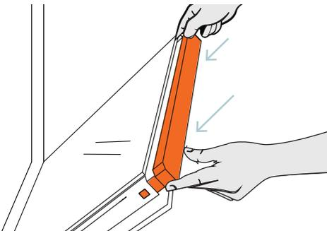
4. Push the cover back onto the top of the door until you hear the buttons click.
