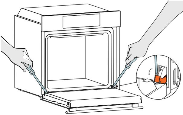
1. Open the door fully and use a screwdriver to rotate the hinge locks outwards, then carefully lift the door off and place it on a soft, level surface.
