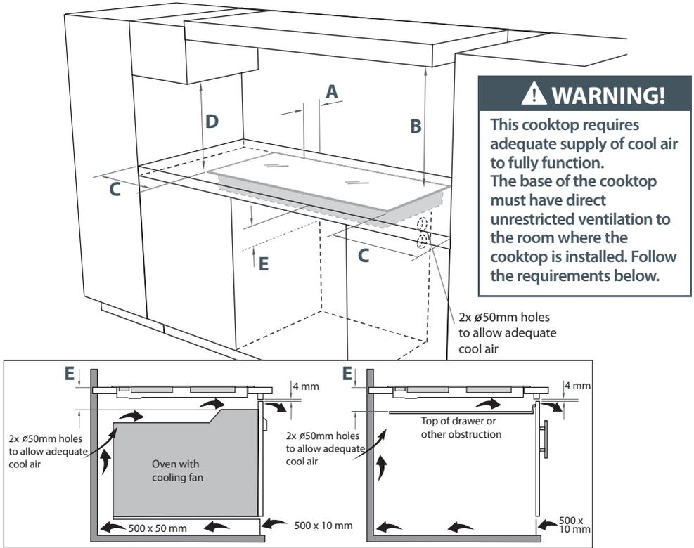
Fig. 1 Minimum clearances and ventilation requirements - oven installed below cooktop
