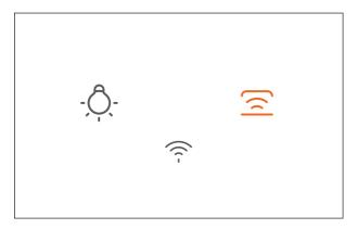
2. On the rangehood press and hold for 3 seconds until the HOB-TO-HOOD button until the icon beeps and flashes 0.5s on/off.
