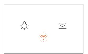
2. The Wi-Fi icon light flashing means the device is attempting to connect to WI-FI/APP. Follow the instructions in the app to complete the connection. Once connected the Wi-Fi icon will stay illuminated.
