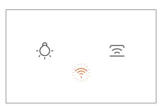
2. The Wi-Fi/App icon light will continue flashing, after 15 minutes the connection will then disconnect, and the Wi-Fi/App light will turn off.
