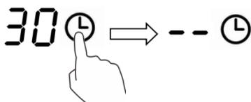
5. When the time is set, it will begin to count down immediately. The display will show the remaining time and the timer indicator will flash for 5 seconds.
