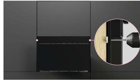
Secure the drawer using the four 7/8" (22mm) screws supplied.
