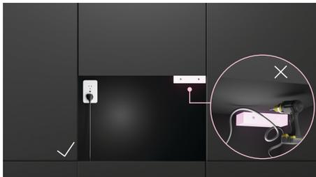
Take care to avoid electrical wiring and plumbing when securing.
