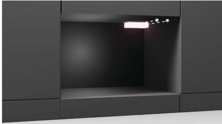
Install the anti-tip block into the cabinetry 14 13/16" (377mm) above cabinetry floor level. Ensure the screws are fitted into wood or metal for stability.
