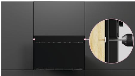
Open the drawer. Using the four holes on the drawer as a template, pre-drill the cabinet using a 1/16" (1.6mm) drill bit.
