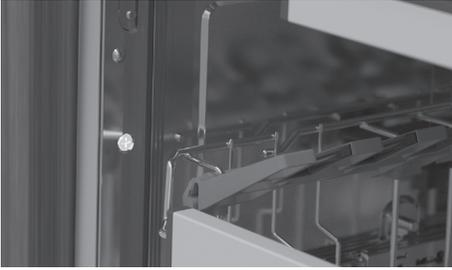
Loosely fit 2 x side fixing screws.
