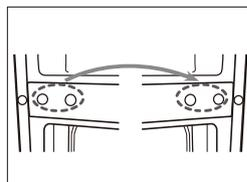
6. Unscrew bottom hinge. Then remove the adjustable feet from both side.
