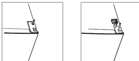
Unplug the temperature sensor from inside the top hinge cover and put the sensor back into the unit as shown below. Remove the door carefully and safely place to protect it from damage.
