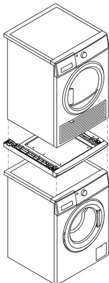
**To ensure stacking stability a stacking kit MUST BE USED between the products and fitted correctly to the washing machine and dryer, as per the stacking kit instructions.**
