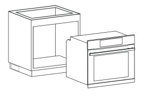
1. Lift the product into the cavity, align it with surrounding cabinetry and appliances.
