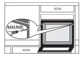
3. Secure the oven to the cavity using the 4 x #3.5x25 screws provided.
