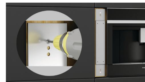
Fit the bracket into place using the supplied screws. Repeat on opposite side.
