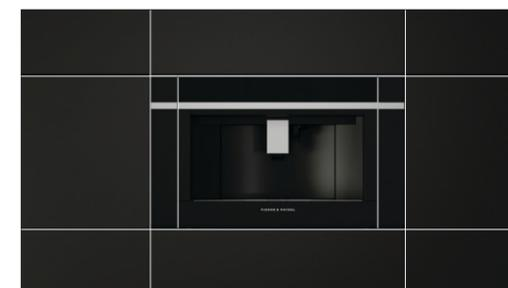
Check the alignment of both trims. If adjustments within  $\pm 1\text{mm}$  are required, remove the trim and adjust the bracket. If further adjustments are required, remove the trim and bracket. Return to step 5 and repeat the process with a new set of holes.
