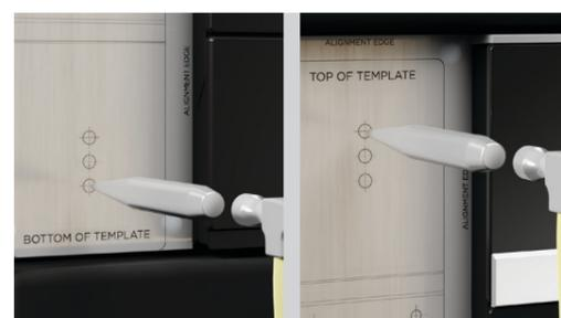
Punch one upper and one lower hole using the locations marked on the template. Note that three sets of holes are provided and not all holes need to be drilled. Drill pilot holes and remove template.
