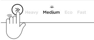
With your DishDrawer™ Dishwasher connected to your Wi-Fi network, press and hold » for four seconds.
