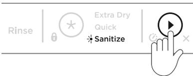
An alert will sound and when the drawer is opened the **SANITIZE** indicator will flash.
