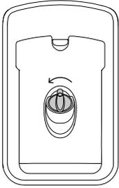
Turn the plug anticlockwise and remove.
