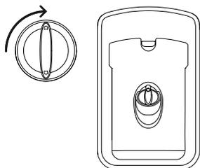
Refit the cap, turning clockwise until secure.
