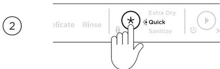
Press ★ to scroll through the wash modifier options. The selected wash modifier indicator will illuminate on the display.
