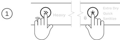
Ensure there is no wash in progress, then open the drawer. Press and hold » and \* together for four seconds.
