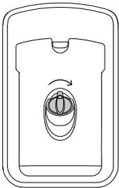
Refit the plug, turning clockwise until secure.
