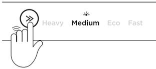
Press » to change the setting within an option. The wash program indicators will display which setting is selected.
