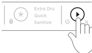
Press ▶ to start the wash and close the door within 7 seconds.
