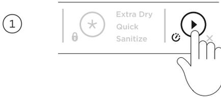
Press and hold ▶ to set the delay start time. Each tone indicates a 1h delay.
