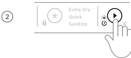
⌚ will illuminate and a tone will sound to indicate each hour of delay. Close the drawer. The wash will start when the delay time is over.
