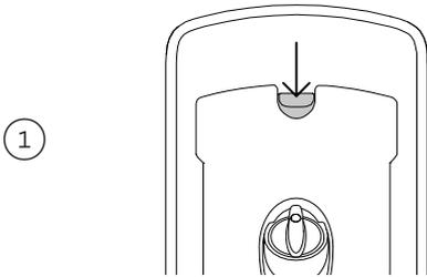
Press the latch down to open the dispenser. Check that the dispenser is empty and dry.
