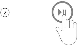
Touch ▶||. The machine will automatically fill to the correct water level for the load, for both phases of the wash.
