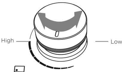
③ After the burner has lit, keep the dial held down for three more seconds (a), then release.
