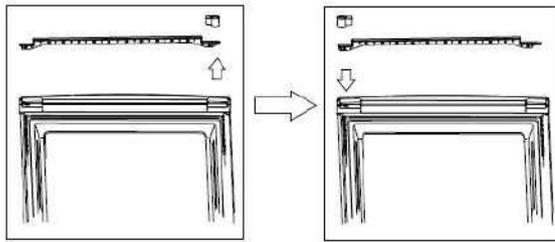
8. Install the upper door, fix the upper door hinge onto the cabinet.
