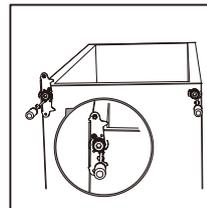
6. Make the middle hinge reverse the direction 180°, then transfer it to the left property position. Make the middle hinge pin in the upper hole of the lower door, then tight the screws.
