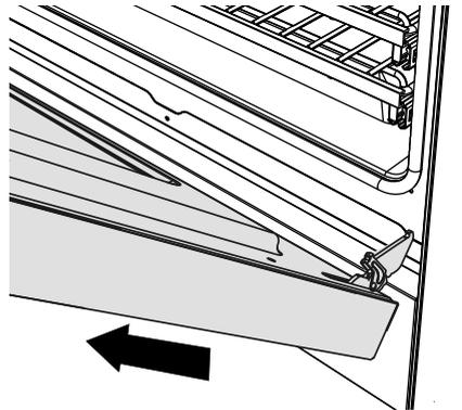
④ Disengage the hinges and remove the door. Place on a protected surface.
