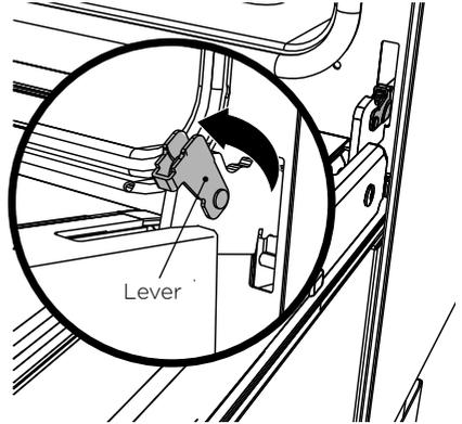
② Open the levers fully on both sides.
