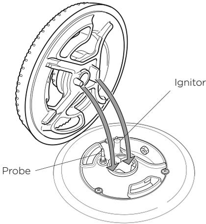
Correct positioning of flame spreader - dual burner
