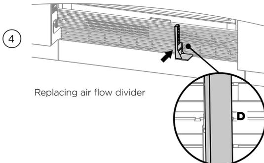
Replacing air flow divider
