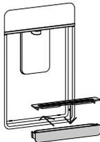
Securely clip the two halves together.
