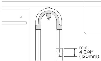
Pull both hoses through the support guide and rest in standpipe. Ensure the drain hose does not extend into water retained in the trap; an air gap is required to prevent waste water from siphoning back into the tub.
