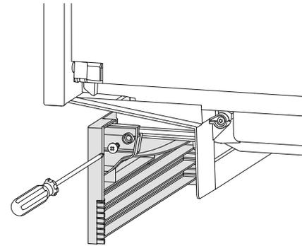
Slide toe kick onto the mounting rails
