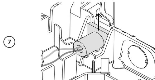
⑦ Safely cut the cord from the inside **and outside** of the product to remove the cord.
