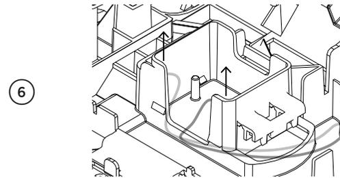
⑥ Unscrew the Live, Neutral and Earth wires as shown.
