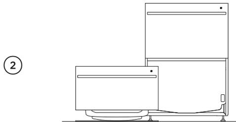
② Lift the drawer off the runners and carefully set aside on a protected surface. Push runners back in. Take care not to pull drawer out too far to prevent any strain on the hoses. Where possible, protect the base of the tub to prevent damage.
