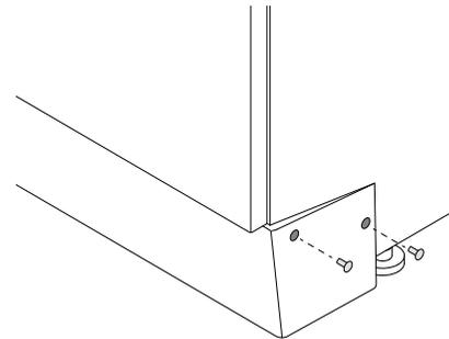
Secure toe kick to the Dishdrawer using the supplied pins.
