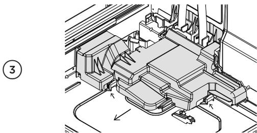
③ With a flat-bladed screwdriver, push in the clips and slide out the access cover.
