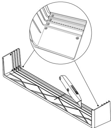
On a protected surface, carefully score down both corners to the desired cut-off point and snap to remove the excess.
