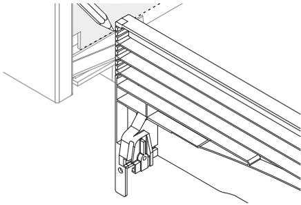
Measure toe kick height. Where the toe kick meets the bottom of the tub is the recommended cut-off point.
