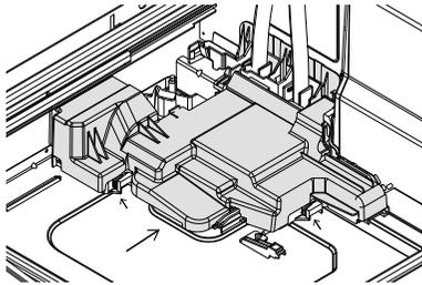
Refit module cover before sliding the access cover back into place, ensuring the 2 clips shown are fully locked.
