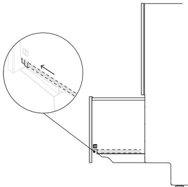
Refit the drawer back onto the runners, ensure both runners are extended halfway before lowering the tub. Slide the runners forward to engage.
