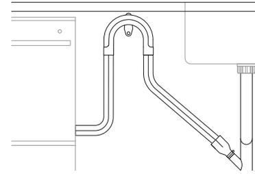
Pull both hoses through the drain hose support before threading the wire clips on to the hoses and fitting to the supplied hose joiner. Secure using the wire clips. Ensure hose is routed straight to the joiner, removing excess drain hose if necessary. Do not shorten the inlet hose. Unplug or drill out the waste tee before securing joiner to sink trap or waste tee.
