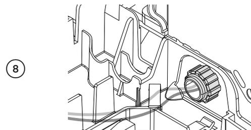
⑧ Fit a suitable cable clamp for the conduit through the metal knockout. Ensure wiring is routed through or under under housing ribs.
