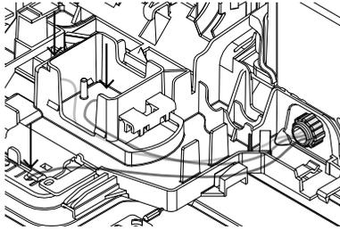
Screw down the Live, Neutral and Earth wires correctly.
