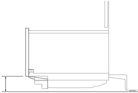
Measure the distance from the floor to the base of the lower door panel. Refer to the table below for the recommended cut location.
