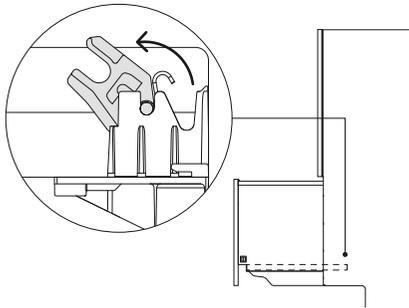
Before refitting the drawers, ensure the hoses are not twisted and all latches are facing forward.
