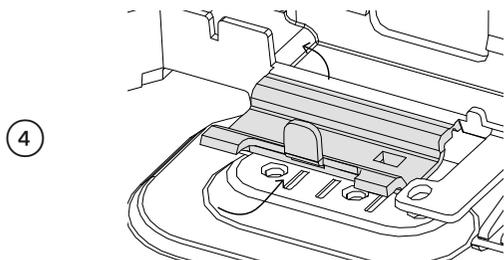
④ With a screwdriver, unclip the plastic harness cover and hinge open.
