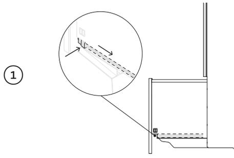
① Open the lower drawer and press both locking tabs back to release.
