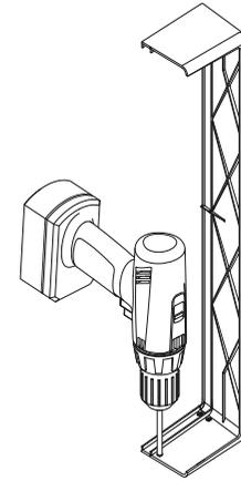
Punch or drill out the two mounting holes with a 5mm drill bit on each side of the toe kick as shown.
