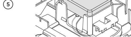
⑤ Slide the terminal block cover sideways to unlock and hinge open to access the terminal block.
