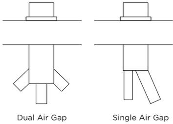
Install your Air Gap Kit to the benchtop. We recommend using a Dual Air Gap Kit. Refer to 'Plumbing & electrical connection' for minimum install heights.
