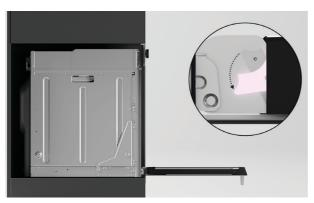
**3.** Push each locking lever down and lock into place.
