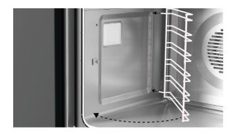
1. Slide the prongs into the holes. Ensure the rack sits flush against the side of the oven.
