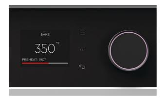
4. Adjust the temperature if needed, then press the dial. Press ••• to set automatic cooking if required. For more information refer to 'Cooking options.'
