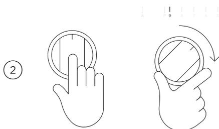
Push in and turn both control dials for the selected cooking zones clockwise to the highest heat setting (9).
