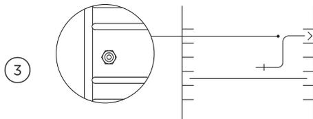
Place food in the oven and plug the probe into the socket inside the oven, on the right hand side.
