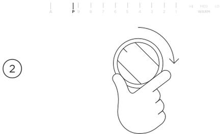
From this setting, turn and hold the dial at **P** until **P** appears in the display.
