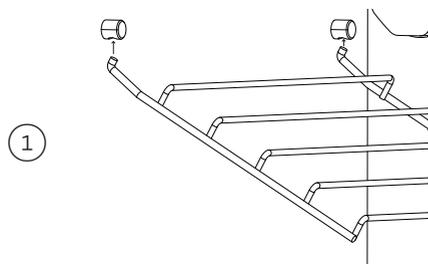
Supporting the side rack from underneath, hold it almost horizontally and locate the prongs into the mounting slots.
