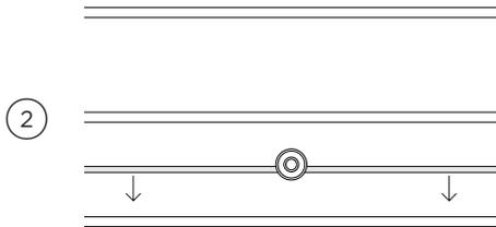
Gently pull down on the retaining wire from underneath the lock stud. The retaining wire will pop out. Unscrew the fixing nut and set aside.
