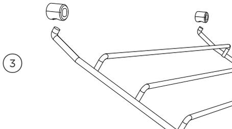
Swing the bottom of the side rack up towards the center of the oven until it is almost horizontal. Slide the prongs at the top out of the mounting slots.
