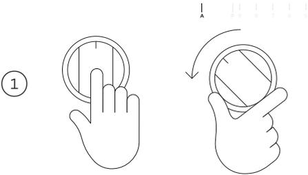
Push in and turn control dial counterclockwise to A. Hold dial at A until **A** appears in the cooking zone display.
