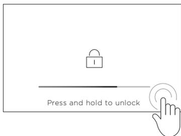
Press and hold anywhere on the screen until the bar fills and the oven unlocks.
