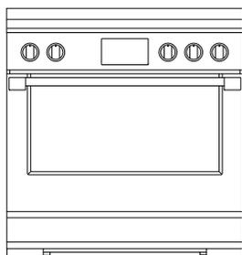
Close the oven door ensuring that when closed, the door is vertical and parallel to any surrounding cabinetry.
