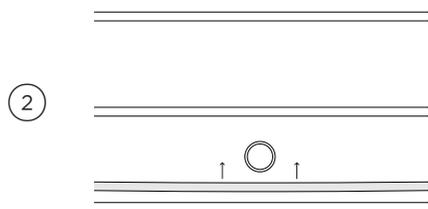
Ensure the prongs are fully inserted into the slots, then lower the side rack carefully and gently push the retaining wire underneath the lock stud.
