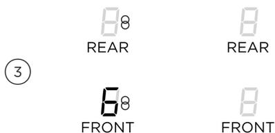
Turn both dials to P and hold until 8 appears in the displays. The front cooking zone display will show the heat setting.
