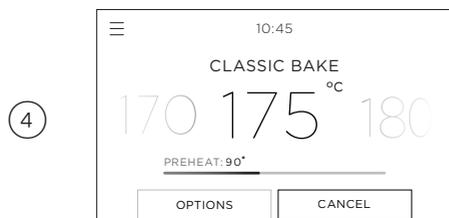
When the oven has reached the set temperature, a tone will sound and the bar will disappear.
