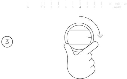
To adjust the heat level during cooking, turn the dial clockwise to any heat setting between **9** and **1**.
