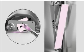
Remove the glass light bulb cover. Using a small flat-head screwdriver, twist and lift the retainer clip to unlock, then remove the glass.
