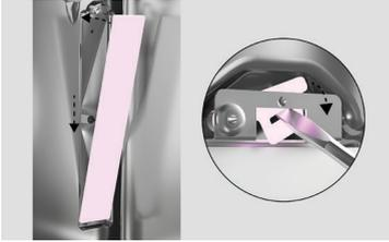
Replace the cover and twist the retainer clip back into place to secure.
