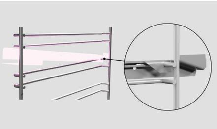
Ensure the rear tags are hooked over the side racks on both sides.
