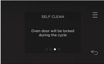
For your safety, the oven door will be locked shut during the cycle. The cycle will not start until the door is properly closed.
