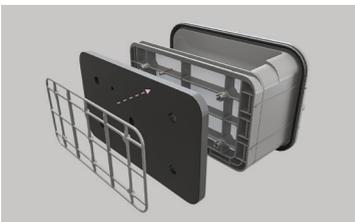
Replace the foam and secure with the bracket.
