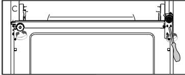
c Unscrew the bottom hinge. Change the bottom foot from current position to opposite side.
