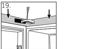
19. Replace faceplate and cover, fix it with the screws and reinsert the fixation (see fig. 3).
