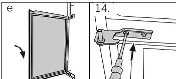
e Lift the lower door carefully onto the bottom hinge so that the pivot fits into the hinge barrel.
