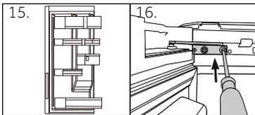
15. Lift the door carefully on to the lower hinge so that the pivot fits into the hinge barrel.
