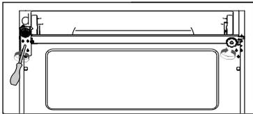
d Take out the new bottom hinge from the accessory bag and screw the new bottom hinge to the other side of the door opening.
