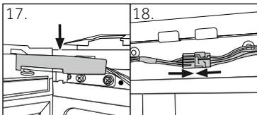
17. Put the connection cable through the hinge cover (delivered in the accessory bag) and put it over the hinge.
