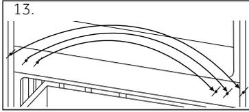
13. Change the positions of the blanking plugs and the screw on the other side.
