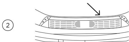
Locate the metal sensors just behind the lint filter.
