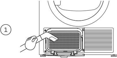
If the surface of the evaporator grid is dirty, clean it carefully with a vacuum cleaner using a dusting brush or a narrow crevice tool. Be gentle and do not bend the fine metal fins.
