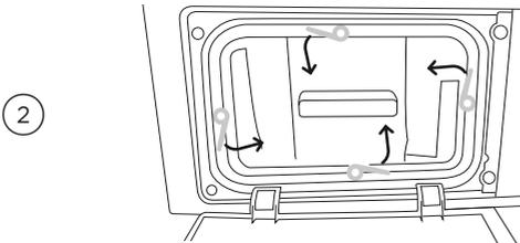
Turn the four condenser lock levers 90° then pull out the condenser filter.
