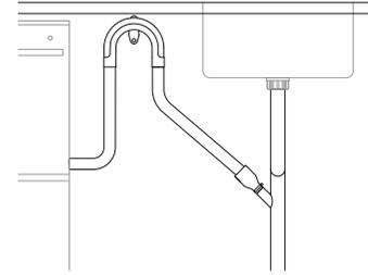
Pull the hose through the drain hose support before threading the wire clip on to the hose and fitting to the supplied hose joiner. Secure using the wire clips. Ensure hose is routed straight to the joiner, removing excess drain hose if necessary. Do not shorten the inlet hose. Unplug or drill out the waste tee before securing joiner to sink trap or waste tee.
