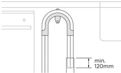
Pull the hose through the support guide and rest in standpipe. Ensure the drain hose does not extend into water retained in the trap; an air gap is required to prevent waste water from siphoning back into the tub.
