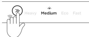
With your DishDrawer™ Dishwasher connected to your Wi-Fi network, press and hold » for 4 seconds.
