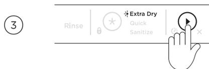
Press ► to save and leave the menu after Wi-Fi is connected. If at any time, you want to exit the menu, press and hold ► to cancel.
