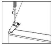
10. Put the hinge cover and the screw cover back.
