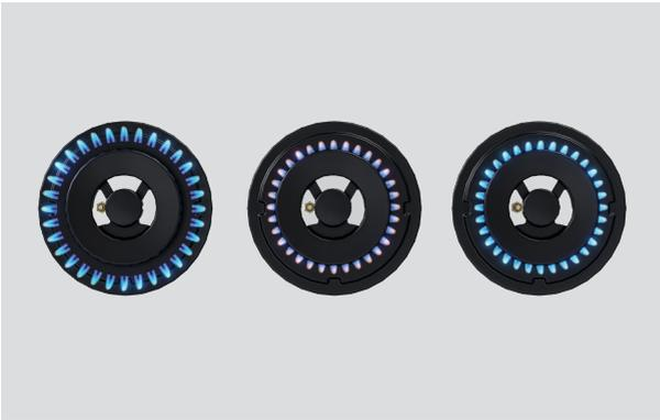
2. Check flames are blue and stable. A yellow flame indicates insufficient air. A noisy flame that lifts away from the burner indicates too much air.
