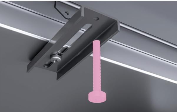
3. Tighten all clamp screws to secure the cooktop to the cutout. Do not overtighten clamp screws. Screws should only make light contact with cutout and joiner strips.
