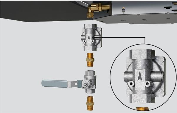
2. Ensure that the regulator arrow points towards the cooktop's inlet pipe, away from the gas supply. Use threading compound on male threads only.
