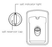
The salt reservoir is located on the inside of the drawer next to the detergent dispenser. It holds up to approximately 350g of salt (actual capacity will vary depending on brand and grain size of salt used).
