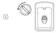
Turn the cap anticlockwise and remove.
