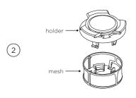
Separate the holder and the mesh by pinching one side of the mesh and pulling.
