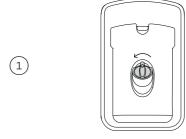
Turn the plug anticlockwise and remove.
