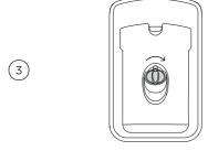
Refit the plug, turning clockwise until secure.
