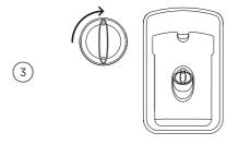
Refit the cap, turning clockwise until secure.
