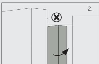
2. If you try to close the left door and the vertical door strip is unbent (2), you should bend it firstly, otherwise the door strip will hit the fixing shaft or right door. Thus a damage to the door slip or a leak will occur.
