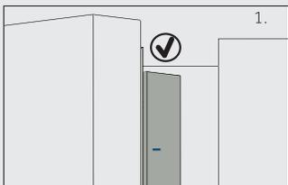
1. When you close the door, the vertical door strip on the left door should be bent inside (1).
