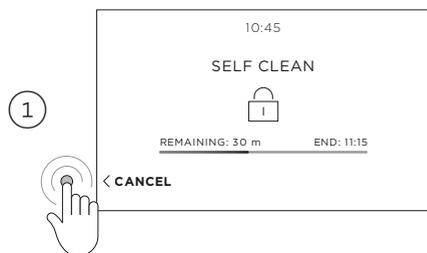
Press the flashing button to the left of the screen at any point during the clean cycle to cancel.
