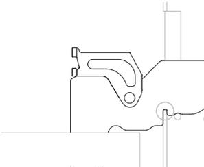
Open the door completely and ensure both hinges are secured by the correct notches.
