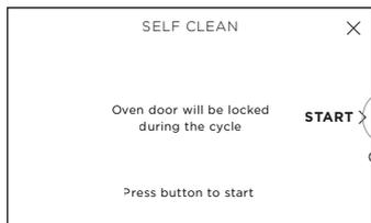
Press the middle button to the right of the screen to start the clean cycle.
