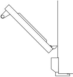
Holding the door at 45°, carefully align the hinge tongues with the hinge slots. Push the door in until you feel the latches locate into position on each side
