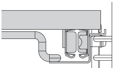
Ensure shelves are positioned on top of the side rack wires instead of between them.
