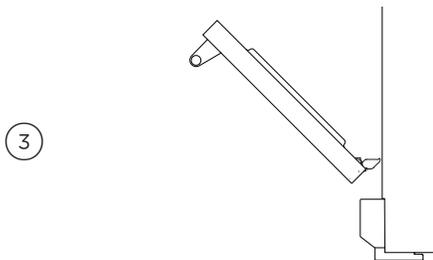
Holding the door on both sides, lift door back up to 45° and carefully pull the door out and away from the hinges.
