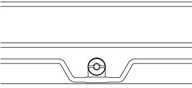
Unscrew the fixing nut holding the side rack in position. A coin may be used to loosen.
