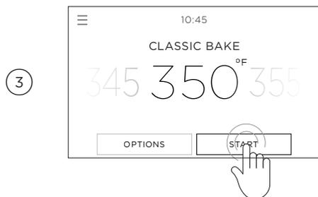
To adjust the preset temperature, swipe left or right or use the dial. Touch **START** to heat the oven and begin cooking.
