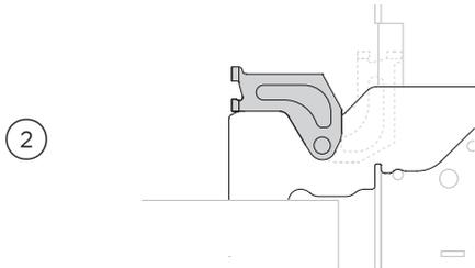
Open the hinge locks fully on both sides
