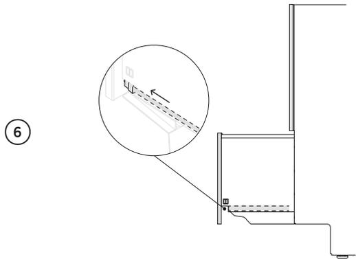
6 Refit the drawer to the runners and clip into place via both locking tabs.
