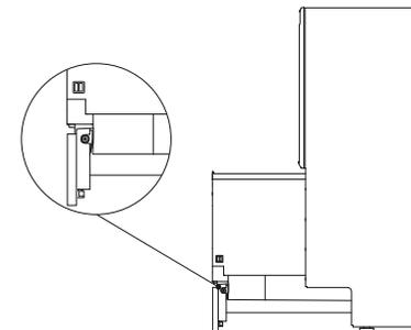
Slide toe kick onto the mounting rails and secure
