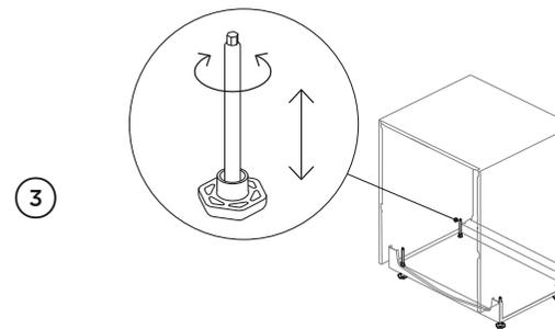
3 Using your hand or the supplied hex socket and a screwdriver, level the DishDrawer™ Dishwasher as required. Rotate clockwise to increase the height of each leg and anticlockwise to lower. It can help to reduce the loading on the feet to assist the adjustment process.
