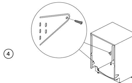
4 Secure to cabinetry via all four fixing locations in the chassis.
