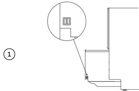
Remove both side pins from each drawer by pulling the pins out towards you.
