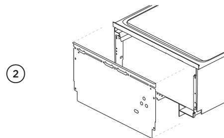
Carefully pull both brackets from DishDrawer™ Dishwasher down and out before unplugging the Knock-to-Pause modules and earth wires.
