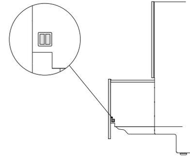
Re-insert the side pins on both drawers and push firmly to secure panels in place.
