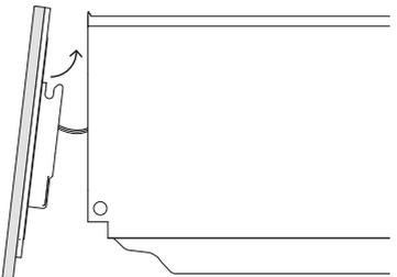
Carefully fit the panels onto the product. When refitting the lower panel, we recommend pushing back the drawer slides as shown on page 13 for access.
