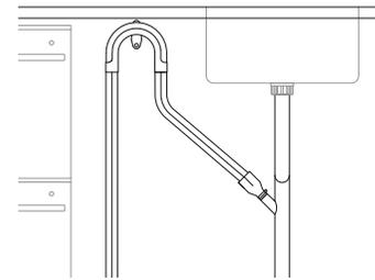
Pull both hoses through the drain hose support before threading the wire clips on to the hoses and fitting to the supplied hose joiner. Secure using the wire clips.
