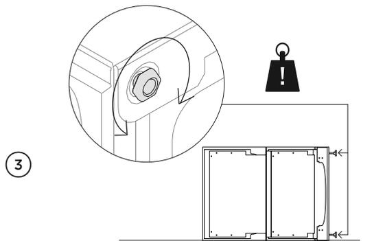
Level the DishDrawer™ Dishwasher by carefully tipping it onto protected surface.
