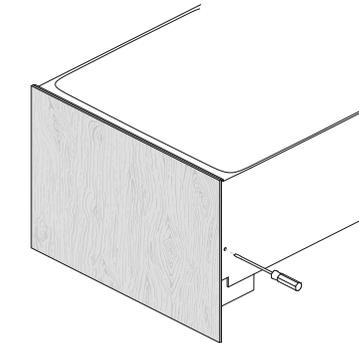
Insert a Phillips screwdriver into the hole above each side pin and rotate to adjust the panel alignment. There is a maximum travel distance of  $\pm 2\text{mm}$ . Repeat for both sides and drawers if required.
