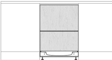
Re-check clearances. **Ensure the minimum clearance gap of 8mm between panels is maintained after all adjustments have been made.**
