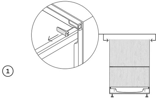
1 Partially open one of the drawers and remove the first screw cover from the trim moulding.
