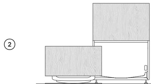
2 Lift the drawer off the runners and carefully set aside on a protected surface. Push runners back in. Take care not to pull drawer out too far to prevent any strain on the hoses. Where possible, protect the base of the tub to prevent damage.
