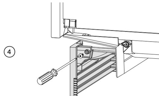
4 Slide toe kick onto the mounting rails and secure
