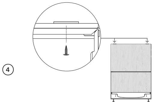
4 If fitted, secure the two top brackets to the cabinetry.
