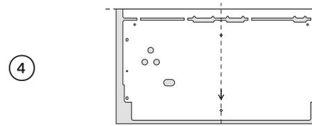
On the back of the lower panel, mark the centre and align the top of the upper bracket with the top of the panel. Secure using a minimum of 3 screws on either side.
