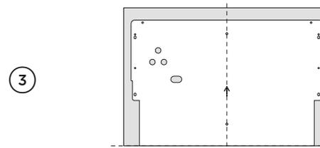
On the back of the upper panel, mark the centre and align the base of the upper bracket with the base of the panel. Secure using a minimum of 3 screws on either side.
