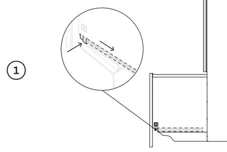
1 Open the lower drawer and press both locking tabs back to release.
