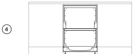
Push the product into the cavity, pulling the hoses through as you push to avoid crushing or twisting them and taking care not to bend the legs.
