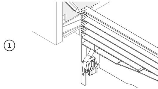
1 Measure toe kick height. Where the toe kick meets the bottom of the tub is the recommended cut-off point.
