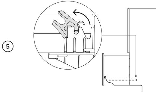
5 Before refitting the drawers, ensure the hoses are not twisted and all latches are facing forward.
