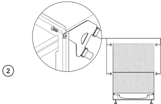
2 Secure to cabinetry via the brackets. Pre-drilling a pilot hole may be required depending on the cabinetry material.
