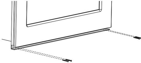
Use the supplied screws to attach the lower trim to the tabs.
