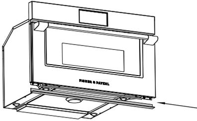
Align the lower trim with the tabs on the base of the oven.
