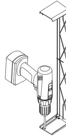
Punch or drill out the two mounting holes with a 5mm drill bit on each side of the toe kick as shown.
