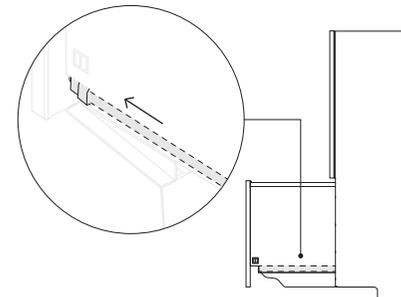
Refit the drawer to the runners and clip into place via both locking tabs.
