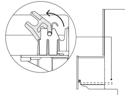
Before refitting the drawers, ensure the hoses are not twisted and all latches are facing forward.
