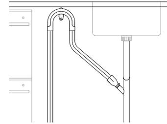
Pull both hoses through the drain hose support before threading the wire clips on to the hoses and fitting to the supplied hose joiner. Secure using the wire clips. Ensure hose is routed straight to the joiner, removing excess drain hose if necessary. Do not shorten the inlet hose. Unplug or drill out the waste tee before securing joiner to sink trap or waste tee.
