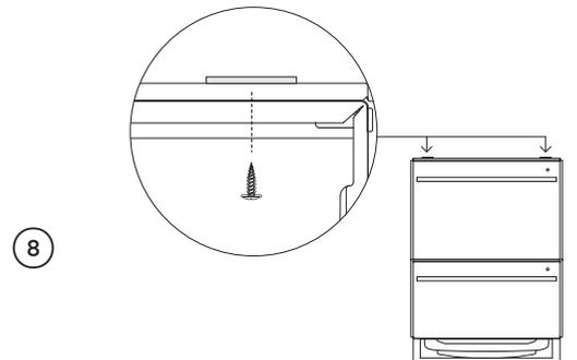
If fitted, secure the two top brackets to the cabinetry.
