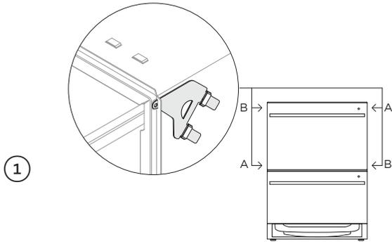
Secure all four side brackets to the DishDrawer™ Dishwasher, aligning bracket A with slot A and bracket B with slot B.
