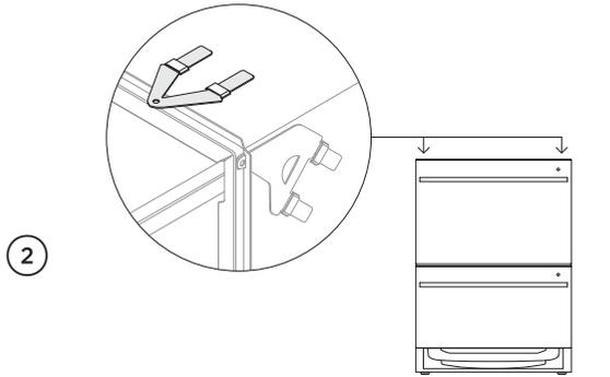
Optionally, fit the two top brackets for additional stability. Ensure the brackets are oriented correctly with the raised locking barbs facing upwards.
