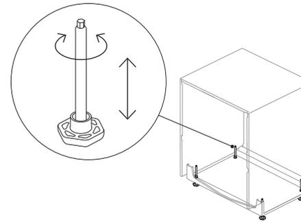
Using your hand or a screwdriver, level the DishDrawer™ Dishwasher as required. Rotate clockwise to increase the height of each leg and anticlockwise to lower.
