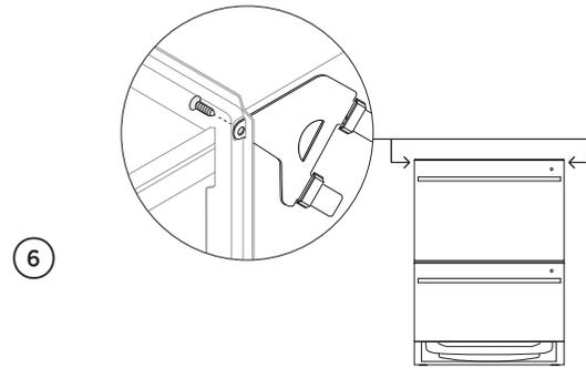
Secure to cabinetry via the brackets. Pre-drilling a pilot hole may be required depending on the cabinetry material.
