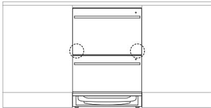
Push the product into the cavity, pulling the hoses through as you push to avoid crushing or twisting them and taking care not to bend the legs.
