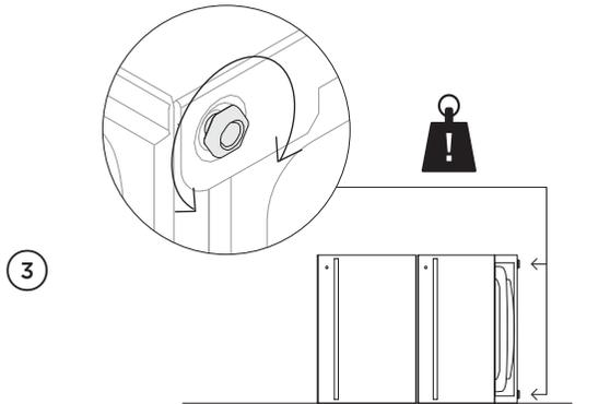
Level the DishDrawer™ Dishwasher by carefully tipping it onto protected surface.
