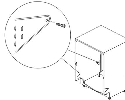
Secure to cabinetry via all four fixing locations in the chassis.
