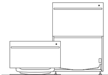
Lift the drawer off the runners and set aside on a protected surface. Push runners back in.
