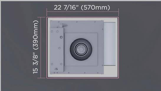
2. Create a 22 7/16" x 15 3/8" (570 x 390mm) cutout in the base of the cavity for the external blower.
