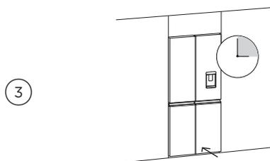
Relocate and install. If the refrigerator has been left on its side for any length of time, leave it standing upright as long as you can (a few hours) before turning on.
