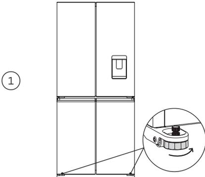
Wind up the feet and carefully ease the refrigerator out of its position. Switch off and unplug.
