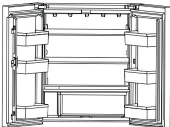
The two full-width cantilever glass shelves are removable and can be repositioned in your refrigerator. The fixed glass shelf can be removed, but not repositioned.
