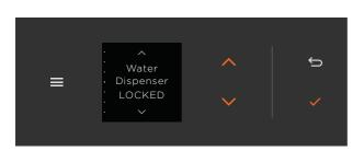
2. Press ✓ or ↑ to scroll to WATER DISPENSER, then press ✓ to lock or unlock the dispenser.
