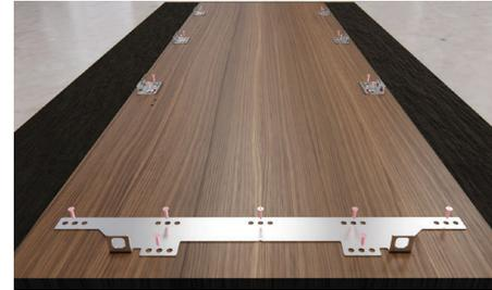
Using the screws supplied in the install kit, secure the door panel bracket using seven screws.
