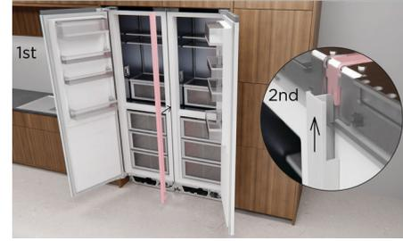
Locate trim between products. Lower trim before pushing in to ensure bottom connector bracket clears the grille. Slide trim up until it slots into the top bracket.
