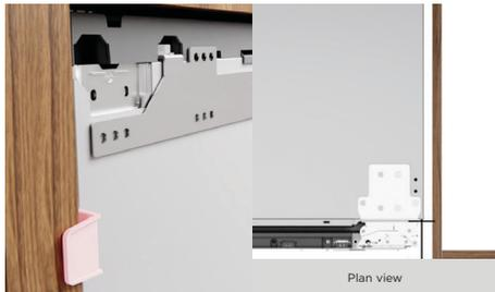
Ensure all depth gauges are flush to the front of the alcove.
