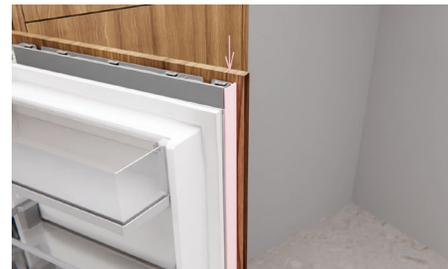
Locate the longer door trim to the non-hinge-side of the product and slide down to clip in place. If a gap is present, remove and readjust the side brackets. Ensure trim does not protrude above the top cover.
