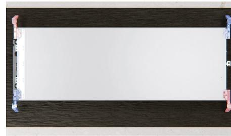
Swap hinges as illustrated. Ensure base of hinge is parallel and tightened securely.
