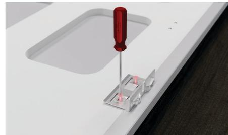
Secure the side brackets using two screws per bracket from the supplied panel kit. Ensure side brackets are fitted tightly and the fasteners are secured straight.
