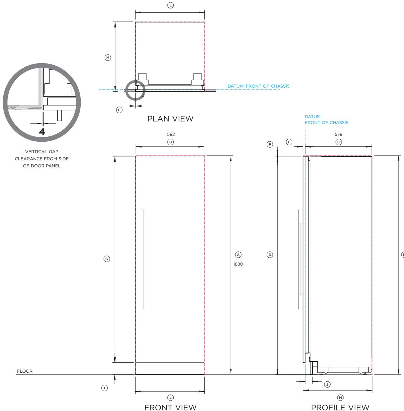
**RS6019S2R1 / RS6019S3RH1 Refrigerator with Stainless Steel Panels RD6019, Handle Kit AHD5RDSF and Stainless Steel Toe Kick Panel AKRS06010**
