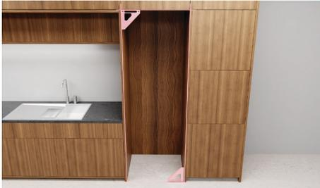
Check alcove is square and is secured to the wall. Ensure front of alcove is square to the top of the alcove and the floor is flat.
