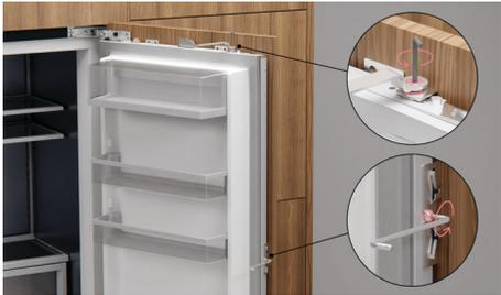
Remove the flow divider and panel bracket before removing all door panel side screws and the M8 washer and nut. Lift panel up and out to remove.
