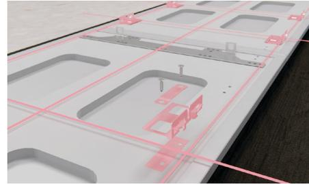
Remove all blue tape from the panel. Align side brackets to the pre-drilled holes based on your hinge orientation. Red labels indicate left hinge installations, blue labels indicate right hinge installations.
