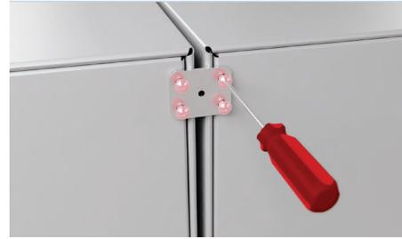
Secure the bracket at the rear top using four screws.
