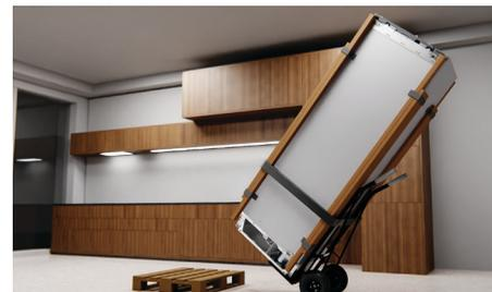
Tilt product onto handtruck and remove pallet. Move product to the installation location. Remove and discard corner posts.
