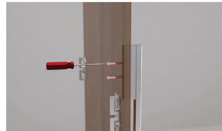
Secure the handle to the panels using 4xM5x25 hex screws per handle. Ensure handle fixings do not interfere with side brackets.
