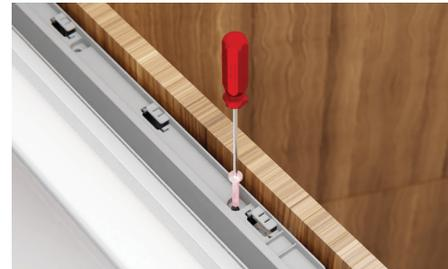
Fit the top cover using two screws. Ensure flat side faces out from the panel.
