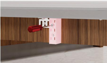
Align flow divider to the screw at the bottom of the door and slot into place. Secure to the door panel using the provided screws.
