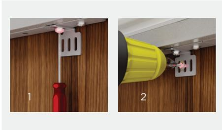
Open the door and loosen the lower bracket screw. Adjust the bracket until it rests against the door panel. Re-tighten the screw and fit an additional screw to secure to panel.
