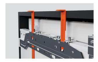
**4.** Raise the height gauge to the top of the cabinet. Align it with the base of the panel above if fitted, or with the base of the door panel if there is no panel above.
