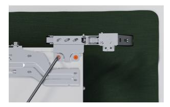
**2.** Carefully remove hinges from door and set aside.
