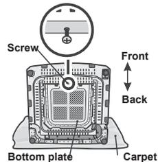
*Note: The washing machine has ventilation openings in the base, the product must not be placed on a carpeted surface.*
