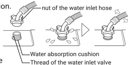
2. Put the nut of the water inlet hose onto the inlet valve thread.
