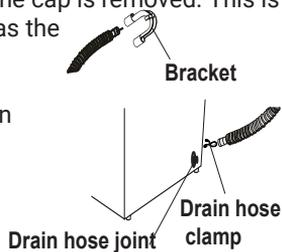
1. The height of the standpipe or tub should be between 0.8 - 1.2 m.
