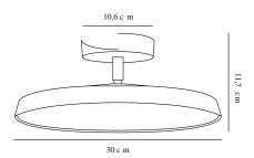
Voltage (V): 230 Volt IP degree if the fixture includes two types of IP degree: IP20 Class (Class I, Class II, Class III): Class 2 (Double isolated) Lampholder type (eg, E27/E14, etc): LED Module Dimmerable: True
